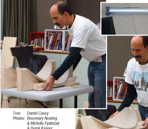
The jig will hold 4 pieces requiring only 2 seems to be connected from inside the pot once it is put together.
