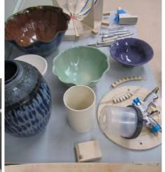
His fluted vessels were made using a set of "support fingers" cut from plywood on the outside.
